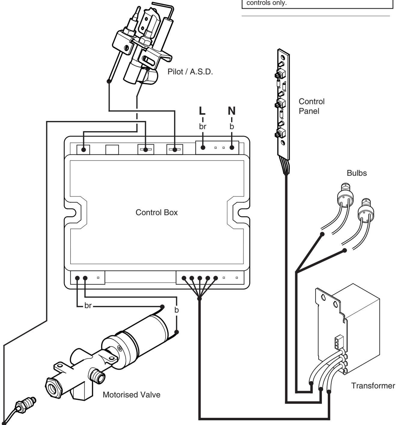
**WARNING:** The appliance must be earthed. The input cable for the appliance should be 0.75mm<sup>2</sup> to IEC Code 27 (heat resistant).
