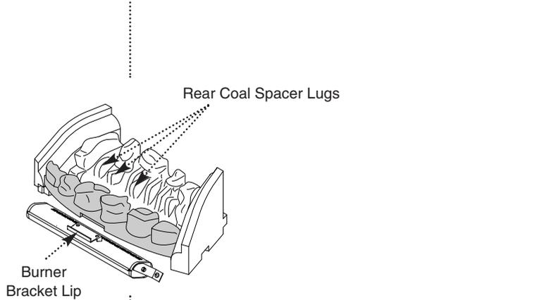
Fig. 27: Diagram showing the rear coal spacer lugs and the burner bracket lip.
