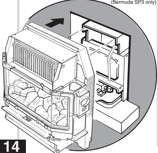
Relocate the flue spigot in the down draught diverter and push the fire backwards as far as possible. Secure the fire to the backing plate using the screws previously removed.
