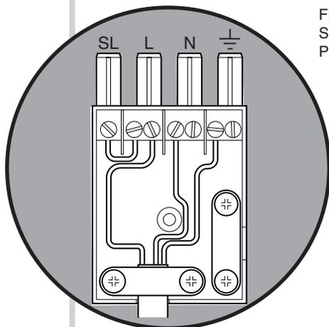
If the firefront does not require a permanent live feed, wire the plug as shown. The loose terminal block can be discarded.
