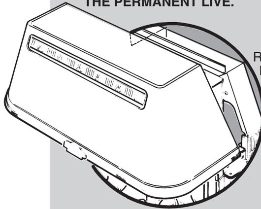
Remove the canopy by gently easing the sides inwards and pulling the bottom edge forward, then lift the canopy upwards and away from the locating lip.
