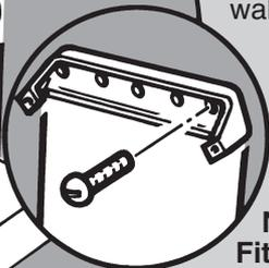
Fix the backing plate in position on the wall using suitable screws.
