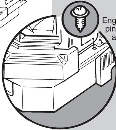
Engage the hearth by guiding the locating pins through the holes in the innercase and sliding forward on the side ledges as far as possible. Fix the hearth in position using the two  $\frac{3}{8}$  in screws in the sides.
