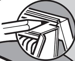
Mark the positions of two suitable fixing holes in the backing plate. **NOTE: Where possible use the top corner fixing hole positions, otherwise space the fixing holes as far apart as possible.**
