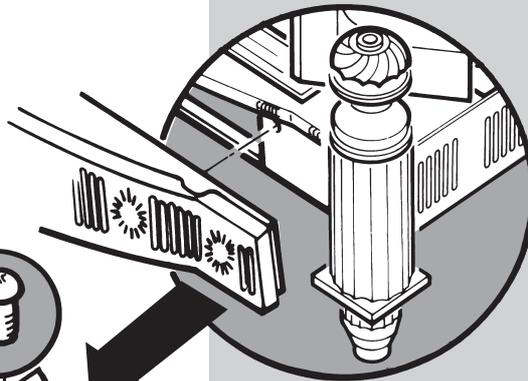
Remove the fender front by pulling forward.
