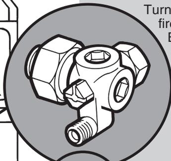
Turn the gas service cock to the boiler and fire position. Purge according to in GB BS 6891 and in IE the current edition of I.S. 813 "Domestic Gas Installations".
