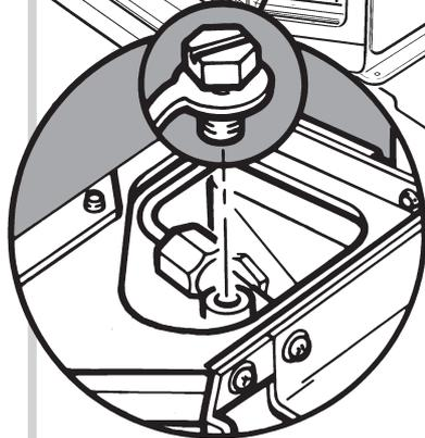
Release the pressure test point sealing screw and connect a pressure gauge in position.
