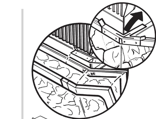
Ensuring that the glass frame is cold, disengage the retaining clamps and lift the frame away.
