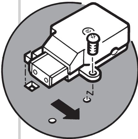
Remove the screw fixing the input socket to the boiler base. Slide the socket to the right, then lift to remove.
