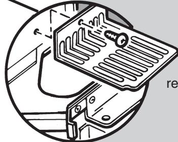
Remove the electrical cover on the right hand side of the chassis by removing the fixing screw.
