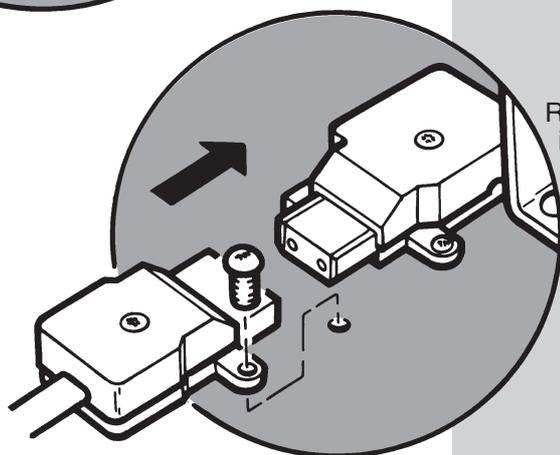
Reconnect the controls connection plug to the input socket and again, fix in place with the securing screw.
