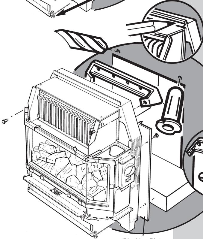
Remove the fire unit from the hearth and remove the backing plate from the fire chassis by removing the two screws holding it in position. Retain the screws.
