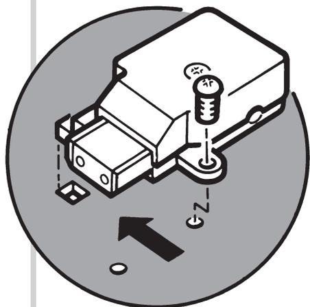
Refit the input socket assembly to the boiler base and fix in place with the securing screw.
