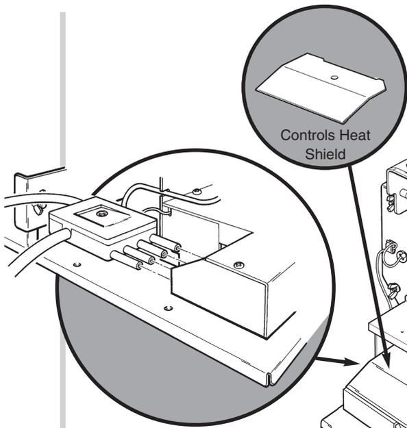
Remove the controls heat shield from its retaining clips.
