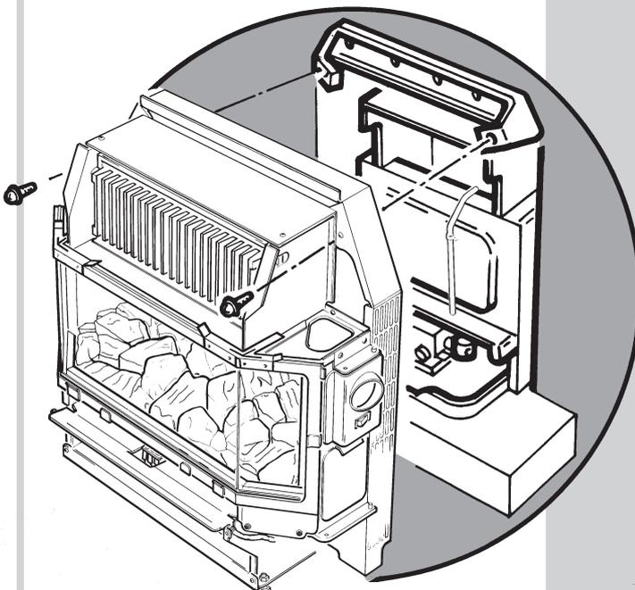
Remove and retain the two screws fixing the chassis to the backing plate. Pull the fire forwards until the flue spigot is clear of the boiler canopy and lift away.
