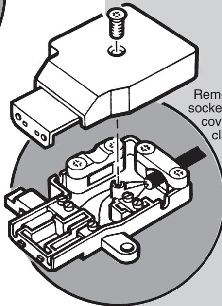
Remove the screw fixing the cover to the socket housing and remove the plastic cover, revealing the terminals and cable clamps and boiler wiring.
