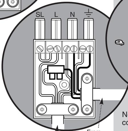
If the firefront being installed is equipped with either lighting effects or lighting effects and electronic ignition the plug must be wired as shown:
