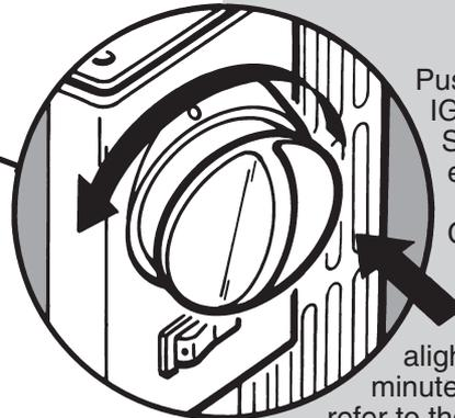
Push in the control knob, turn to the IGNITION position (★🔥) and hold in. Sparking will commence at the ignition electrode and the pilot will ignite.
