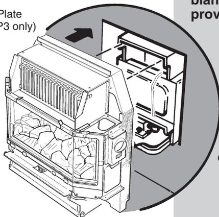
Relocate the flue spigot in the down-draught diverter and push the fire backwards as far as possible. Secure the fire to the backing plate using the screws previously removed
