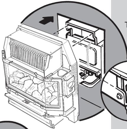
Take the backing plate and fix it to the fire unit with two of the  $\frac{5}{16}$ in screws provided. Locate the flue spigot into the down-draught diverter on the boiler unit. Push the fire backwards until the backing plate touches the surround or wall face.
