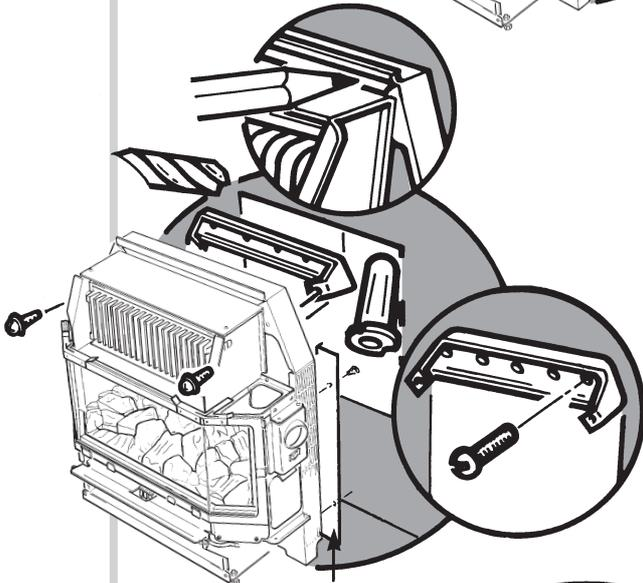
Mark the positions of the available fixing holes in the backing plate. **NOTE: Where possible use the top corner fixing hole positions, otherwise space the fixing holes as far apart as possible.**
