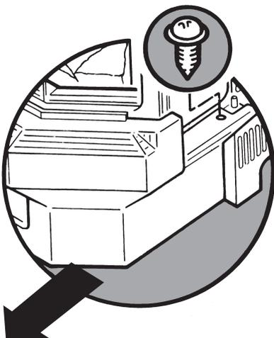
Remove the hearth by removing the fixing screws and sliding the hearth assembly forward and away from the chassis.
