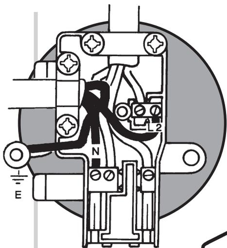
From the plug and cable connection supplied with the fire unit, the following connections should be made, making sure that the appropriate cable clamp is used to hold the cable firmly.
