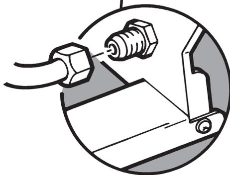
Disconnect the fire supply pipe from the fire inlet.
