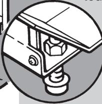
Level the fire by adjusting the front feet (check using a spirit level).
