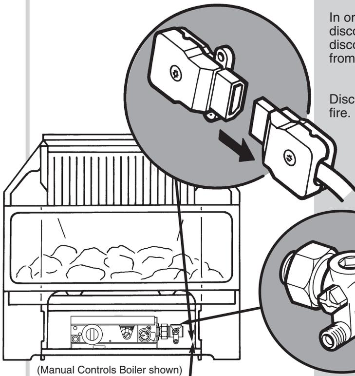
In order to service the boiler unit, the fire must be disconnected and removed at this point. Once disconnected the fire unit may be serviced separately from the boiler.
