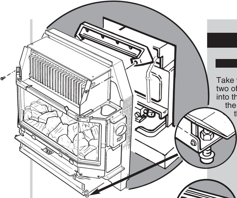
Take the backing plate and fix it to the fire unit with two of the  $\frac{3}{8}$ in screws provided. Locate the flue spigot into the down-draught diverter on the boiler unit. Push the fire backwards until the backing plate touches the surround or wall face. Ensure that the down-draught diverter bottom passes over the controls heat shield.
