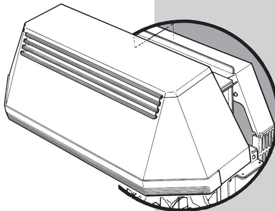
Fix the canopy by guiding the bottom edge onto the door pins and then by tilting the back edge over the locating lip on the innercase. Close the doors ensuring they lock in place.
