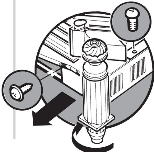
Remove the hearth assembly by removing the fixing screws and sliding it forward and away from the chassis.
