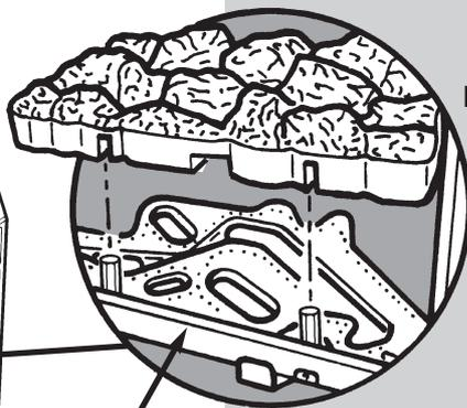
Remove the coal bed by carefully lifting away from the locating pins and place to one side.
