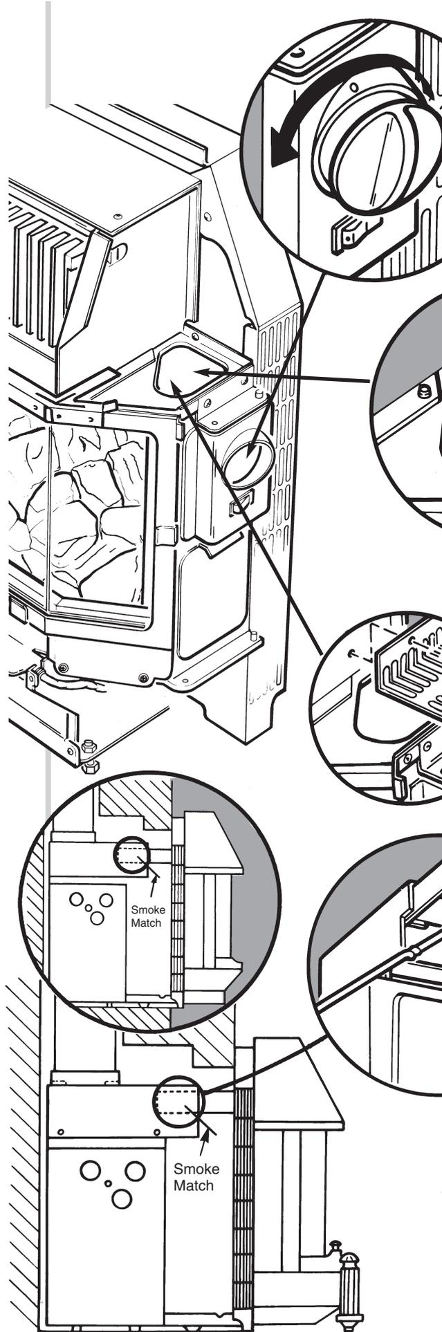
Check the setting pressure at position 4. No adjustment to the setting pressure is possible.
