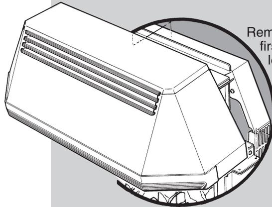
Remove the canopy, firstly by opening the left and right hand side doors, then lift the canopy by the bottom edge upwards and away from the locating lip.
