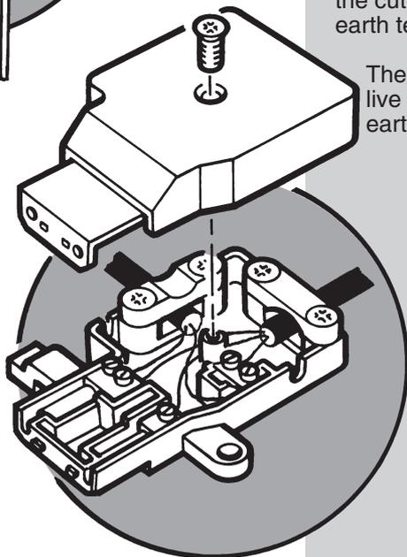
The earth wire should be long enough so that the live and neutral wires will become taut before the earth wire if the cable is pulled.
