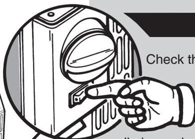
Check the electricity supply to the fire unit by switching on the illumination bulbs. If the bulbs light, switch off and continue with commissioning the fire. If the bulbs do not light, isolate the electricity supply and perform preliminary electrical system checks before proceeding i.e. earth continuity, polarity, resistance to earth etc.
