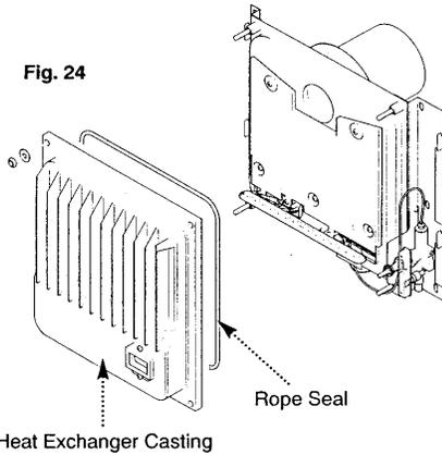
Heat Exchanger Casting
