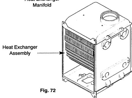
The burner and heat exchanger can be changed after removal of the combustion box door. To change the heat exchanger, the fan and burner must be removed first (see section 13.17 & 13.21).
