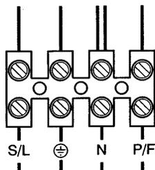
S/L = Switched live to the Boiler from the System Controls.
